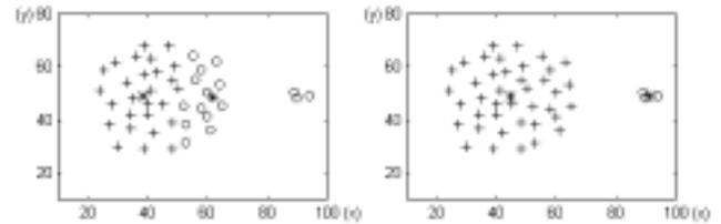
Figure 7: Two partitions obtained by (a)FCM ( $m=1.3$ ) (b)PIM ( $m=1.3$   $\delta = 0.4$ )
