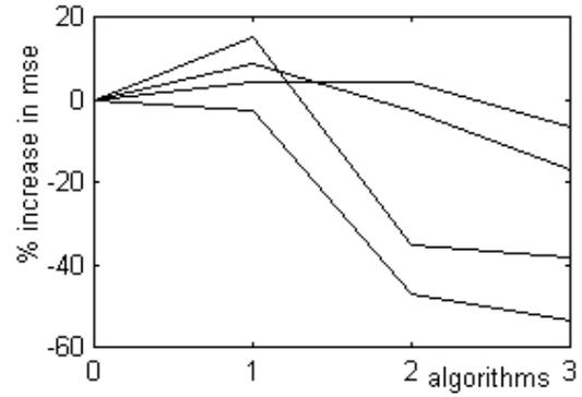
Figure 9: Percentage increase in mse using HVS approach: 0. Reference is the mse after fuzzy quantization(FCM) 1. Quantization with ICS algorithm 2. Error diffusion after FCM 3. Error diffusion after ICS
